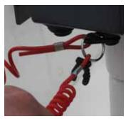
Locate the kill switch and attach the two lanyards as above
