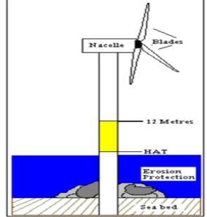
Figure 1 Components of a wind turbine
