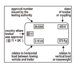
The coupling must be suitable for the vehicle combination and bear an indelible approval mark clearly legible even when it is attached to a vehicle. This mark or label must give certain information about its properties, including the manufacturer's name and part number.
