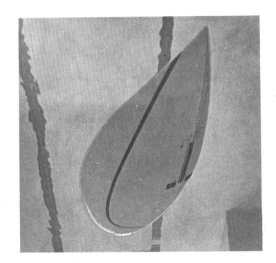
6. In Photo No. 6 the boat is down by the stern and is heeling about 10 degrees. This is an attitude frequently seen under strong planing conditions, where the boat has been allowed to heel a bit, weight is aft and speed may be great.
