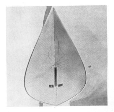
Photo No.1 shows the Finn the way the designer drew it — level both fore and aft and athwartships. And this is the way it should be sailed most of the time. The two squiare patches are the self bailers, one one either side of the after end of the centerboard box. The scuff marks forward of the box were made while launching the boat in the pool, and Yacht Racing magazine certainly hopes its West Coast Editor managed to sand the bottom clean and smooth for the owner.
