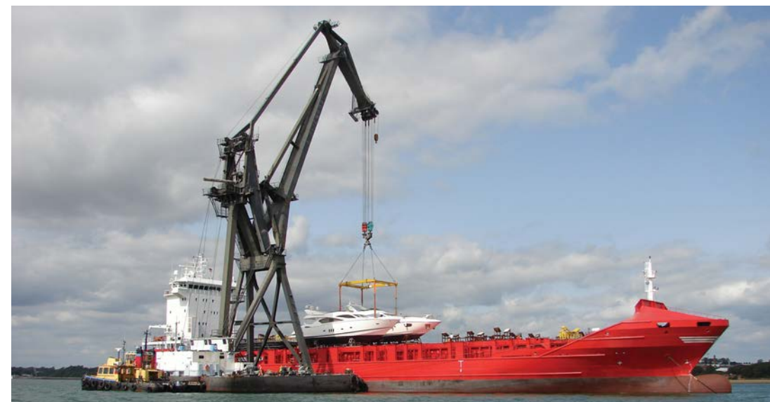
Above: Tandem lift by a geared vessel from water to ship's deck.
