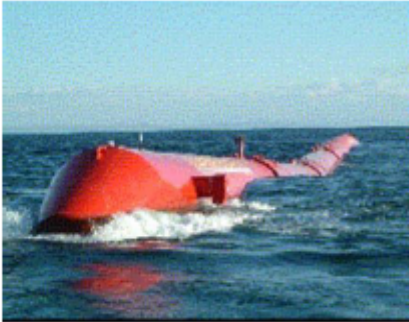
Pelamis Ocean Power Delivery (wave turbine installation) – Recommended colour above the waterline is yellow. (Photos Courtesy Pelamis Wave Power)
