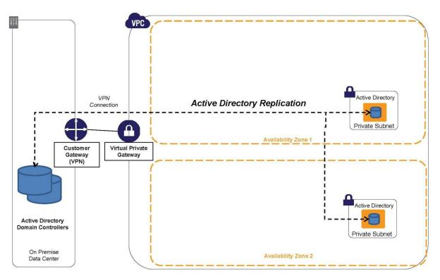
Figure 8: Active Directory Deployment in AWS with Replication
