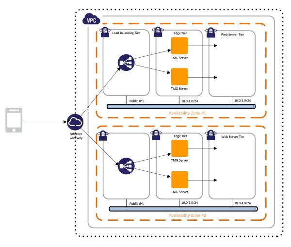
Figure 11: Using Forefront TMG for Threat Protection and Policy Enforcement
