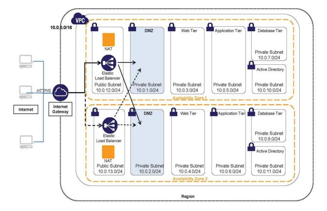
Figure 1 – Isolated environment with full Internet access
