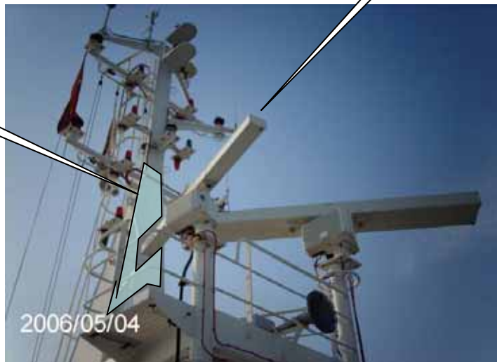
Figure 9: (Above) & Figure 10: (Above Right): Mirror image 'A' generated aboard "FINN FIGHTER" inbound to London. The cause of the image was traced to the forward surface of the rectangular signal mast ('A1' and shaded blue) abaft and immediately to port of the 3cm radar scanner 'B' (left of picture starboard side) below.
