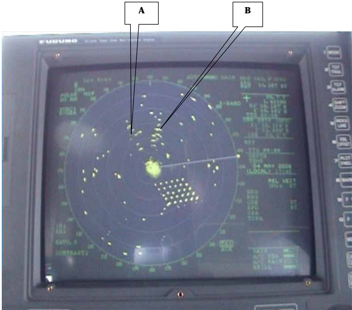
Figure 8: Examples of Incomplete External Mirror Images. Image 'A' is reflected from the Shivering Sands towers and Image 'B' is reflected from an overtaking car carrier.
