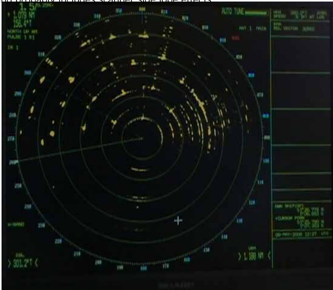
Figure 25: Sector Interference showing to the north
