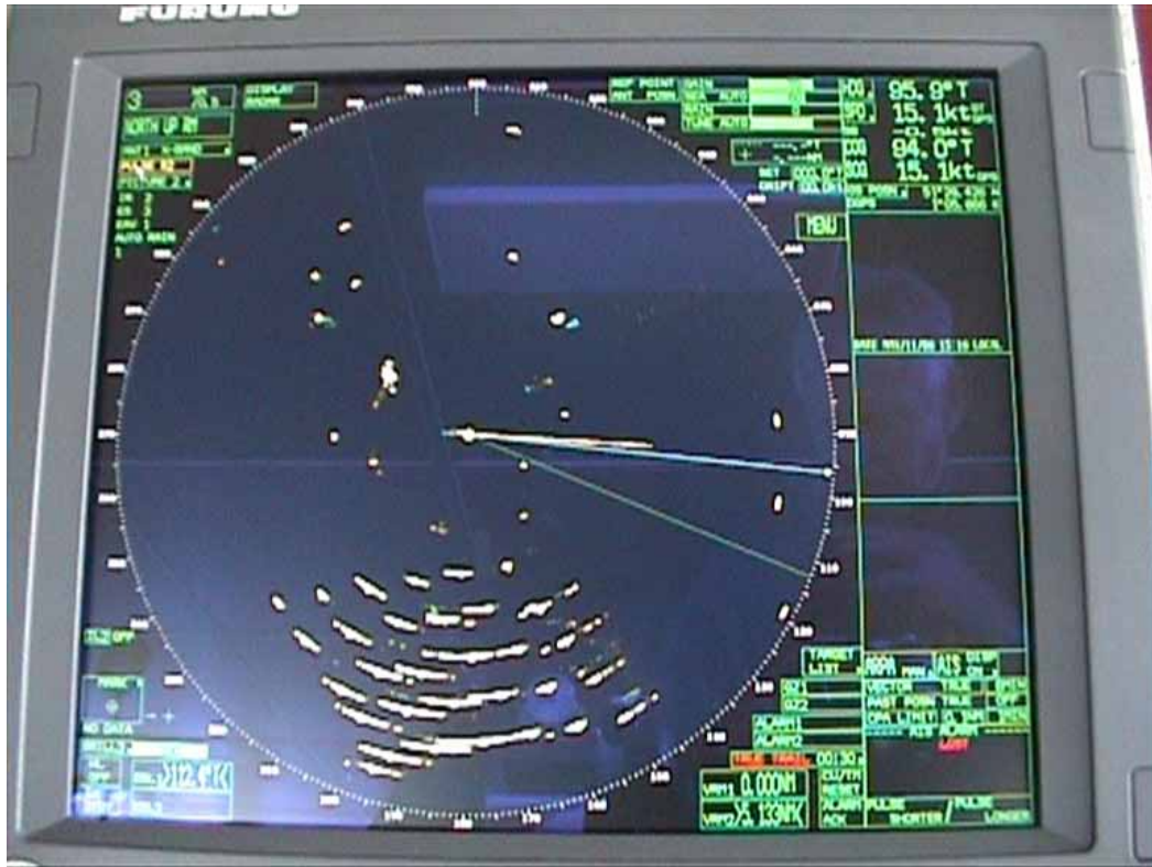
Figure 6: The “OSTSEE” – a Dredger working the Princes Channel, was particularly affected by spurious echoes caused by the many masts around her bridge as well as having athwartships mounted radar scanners.
