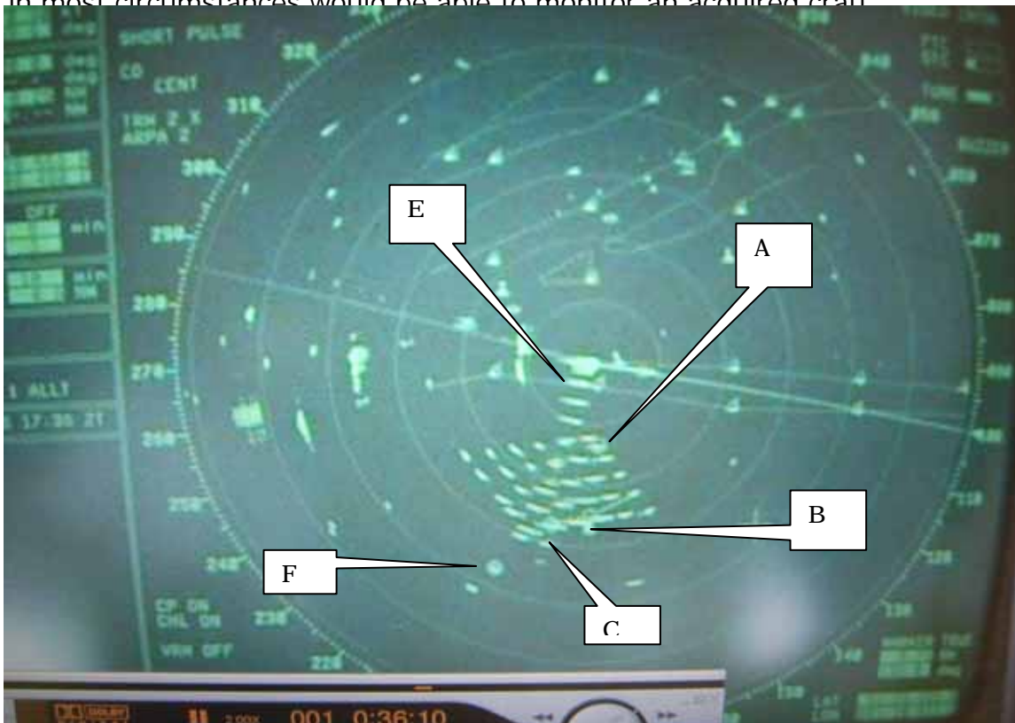
Figure 20: Radar image from "BIRKA CARRIER", outbound from Tilbury; video recording. Small fishing vessel 'A', "MORVEN" 'B' and wind farm Service Vessel 'C' are all visible despite multiple echoes from Car Carrier 'E' between observing vessel and the wind farm. The Spaniard Buoy 'F', used as a reference, remained identifiable throughout. It is also notable that the trial vessel being on the
