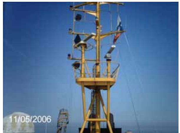
Figure 6: The “OSTSEE” – a Dredger working the Princes Channel, was particularly affected by spurious echoes caused by the many masts around her bridge as well as having athwartships mounted radar scanners.
