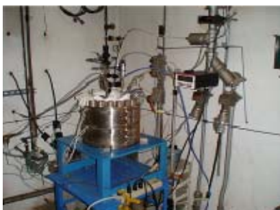
High Pressure & Temperature Flammability Test Set-up in the Pressure Barricade Cell Area
