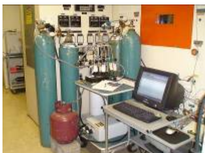
High Pressure & Temperature Flammability Test Set-up in the Pressure Barricade Cell Area
