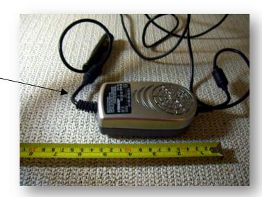
This converter changes 12 volts into 15, 16, 18, 20, 22, or 24 volts DC.
