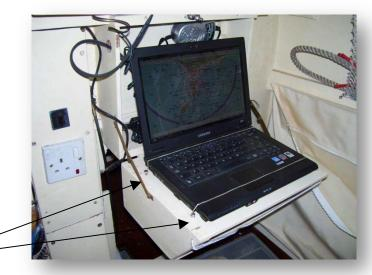
one at the back of the keyboard and one at the front of the keyboard. The lashings are secured to the heads of self tapping screws – which sounds crude – but works.
