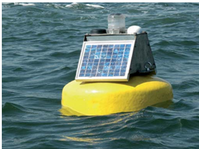
The DataBuoy deployed in Poole harbour monitoring water quality over the oyster beds
