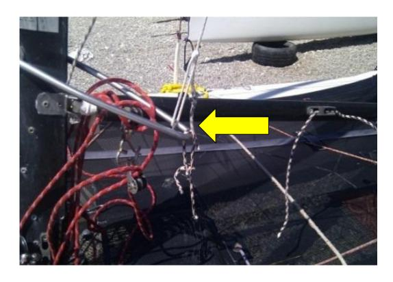
Rotator arm and line that caused the entrapment
