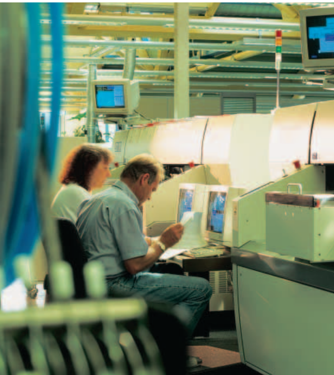
PROGRAMMING OF THE FULLY AUTOMATED EQUIPMENT WITH WHICH UP TO 40 000 ELECTRONIC COMPONENTS PER HOUR CAN BE INSERTED ON PRINTED CIRCUIT BOARDS.
