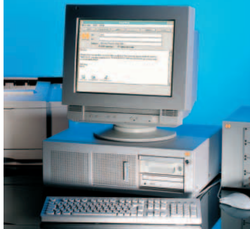
THE HC-6950 EMISSION PROTECTED SECURITY WORKSTATION BY CRYPTO AG OFFERS COMPREHENSIVE PROTECTION AGAINST UNINTENTIONAL EMISSION OF COMPROMISING INFORMATION.
