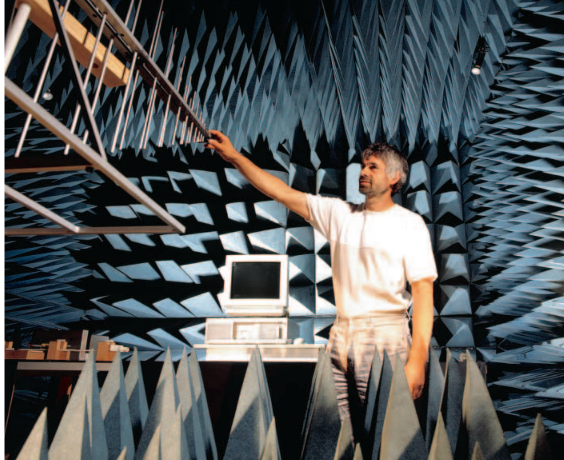
IN CRYPTO'S OWN EMC LABORATORY, OUR EXPERT ANDREAS FOSTER TESTS WHETHER THE EMISSION PROTECTED SECURITY WORKSTATION MEETS THE PRESCRIBED GUIDELINES WITH REGARD TO EMISSIONS.
