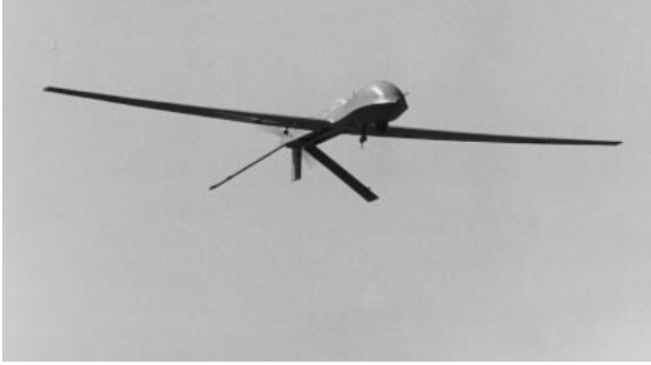
A high-performance unmanned surveillance aircraft (Predator Tier III), now in flight testing.
