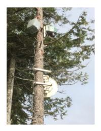
OrcaLab began to experiment with remote cameras in the 1990s and during the NTT Data collaboration was able to show to the world the orcas rubbing from the vantage of two trees above the beach. Step by step, the quality of the video imagery has improved. Prior to 2015, analogue surveillance cameras were used, and in 2016, on the same trees, new higher grade high definition 1080p cameras replaced the 720p cameras Tim had previously installed.
