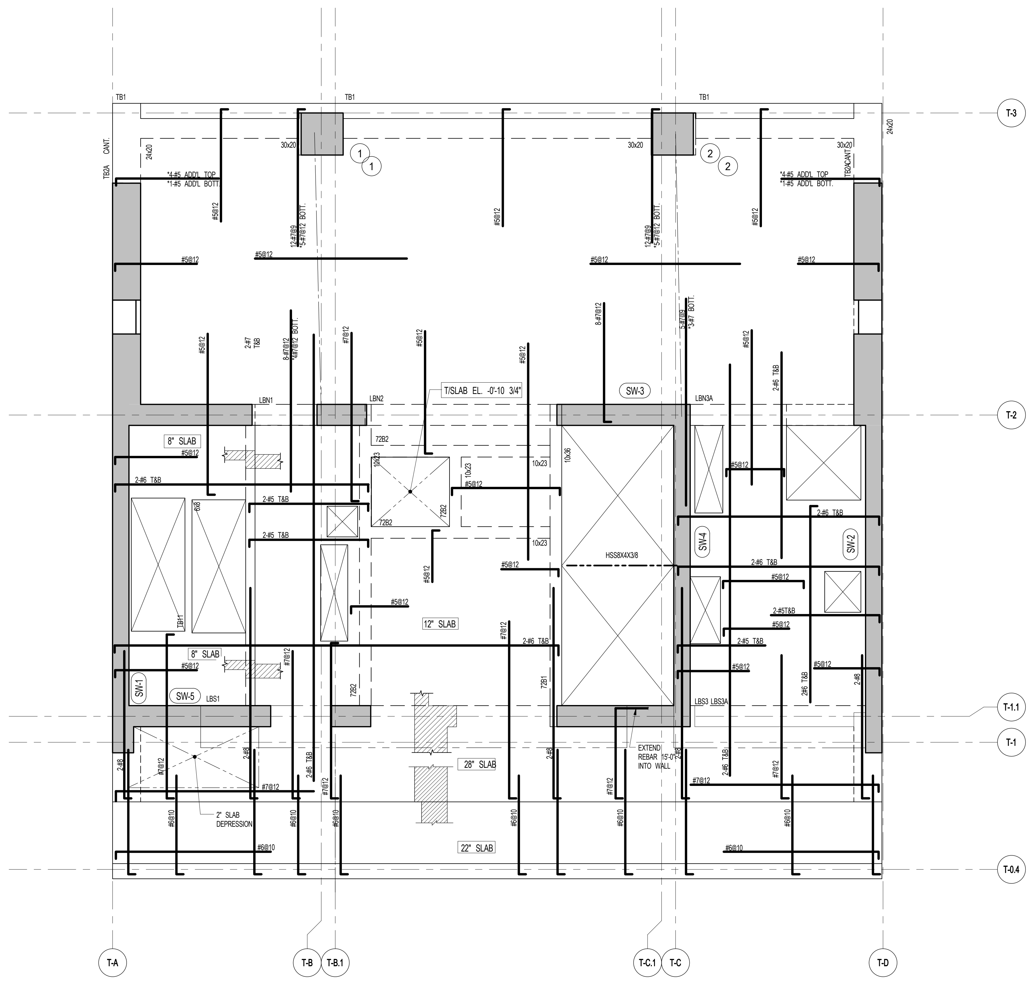
1 74TH FLOOR FRAMING PLAN SCALE: 1/4" = 1'-0" NOTES: 1. TOP OF SLAB EL. SEE ARCH. DRAWINGS. 2. SLAB THICKNESS TO BE 12" UON, THUS E.W. CONTINUOUS FOR 2" SLAB. 3. BOTTOM REINFORCEMENT TO BE #5@12 E.W. CONTINUOUS FOR 2" SLAB. 4. FOR BALANCE OF NOTES SEE DRAWING S-740.
