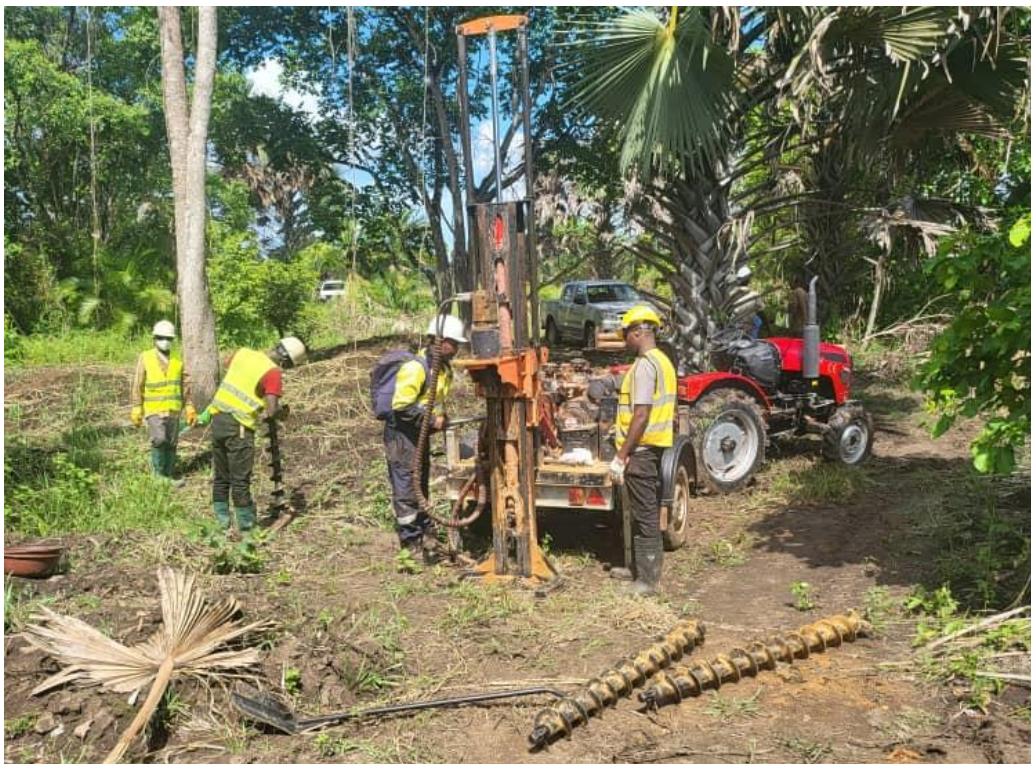
Figure 1: Auger drilling on the Poku Trend, Didievi Project
