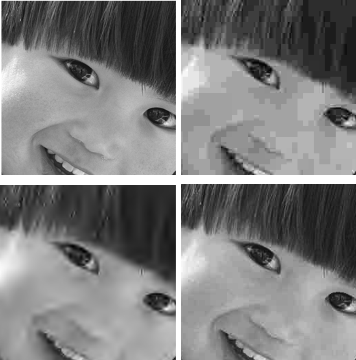
Figure10 – Enlarged portion of the pictorial region of original and reconstructed images at a compression ratio of 70:1. Top left: original; top right: JPEG baseline; bottom left: SPIHT wavelet-based coder; bottom-right: MRC using JPEG+MMR+JPEG without plane subsampling. Portion size is 256x256 pixels.
