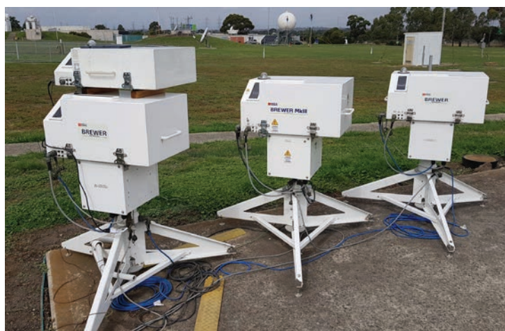
Calibration of Brewer spectrophotometers at the Bureau of Meteorology Training Centre in Broadmeadows, Victoria prior to deployment using the reference instrument from International Ozone Services in Canada (the small instrument on top of the Brewer on the left).
