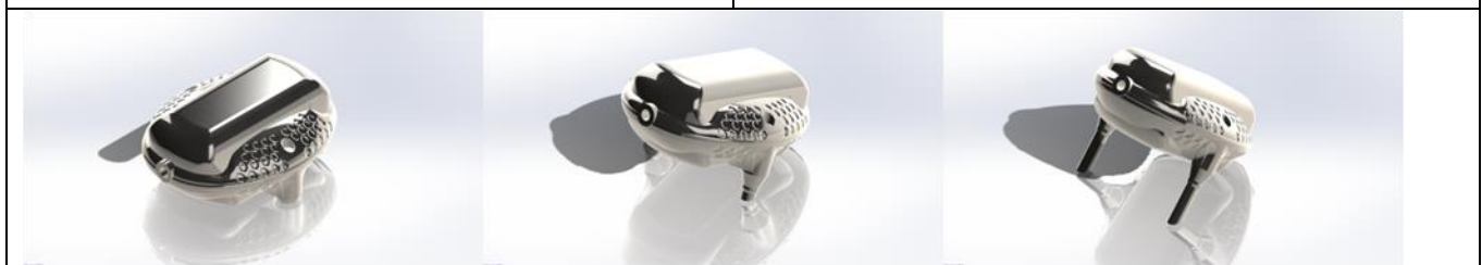
Fig. 18. Top: Drag force (Left) and lift force (Right) at various inclination angles. Bottom: inclination angles of 0° (left), 20° (center), and 40° (right). Flow direction: lower left to upper right.
