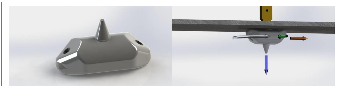
Fig. 5. Computer model of old model AM-240A (left) and force sign convention used for reporting the results (right). Flow is from left to right. The blue, red, and green arrows indicate, respectively, positive lift, drag, and side forces. The clear arrow indicates positive rotation angle.
