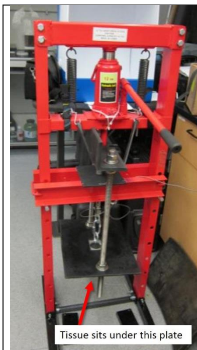
Fig. 23a. Apparatus for dart pull testing.
