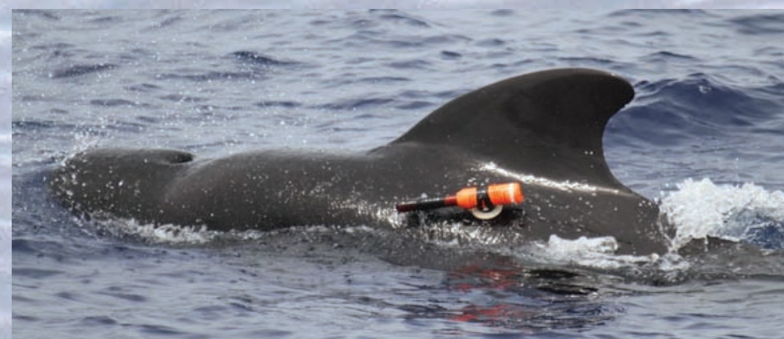
Acousonde 3A acoustic recording tag on short-finned pilot whale, Kona, Hawaii, May 2011. Photo by R. Baird.
