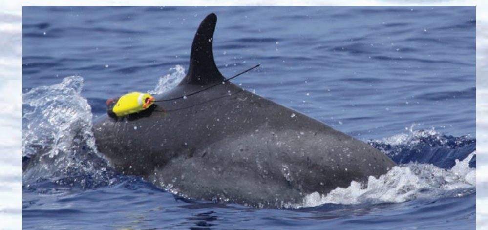
84 s after attachment. The tag has self-aligned with the flow direction. Photo by J. Aschettino.
