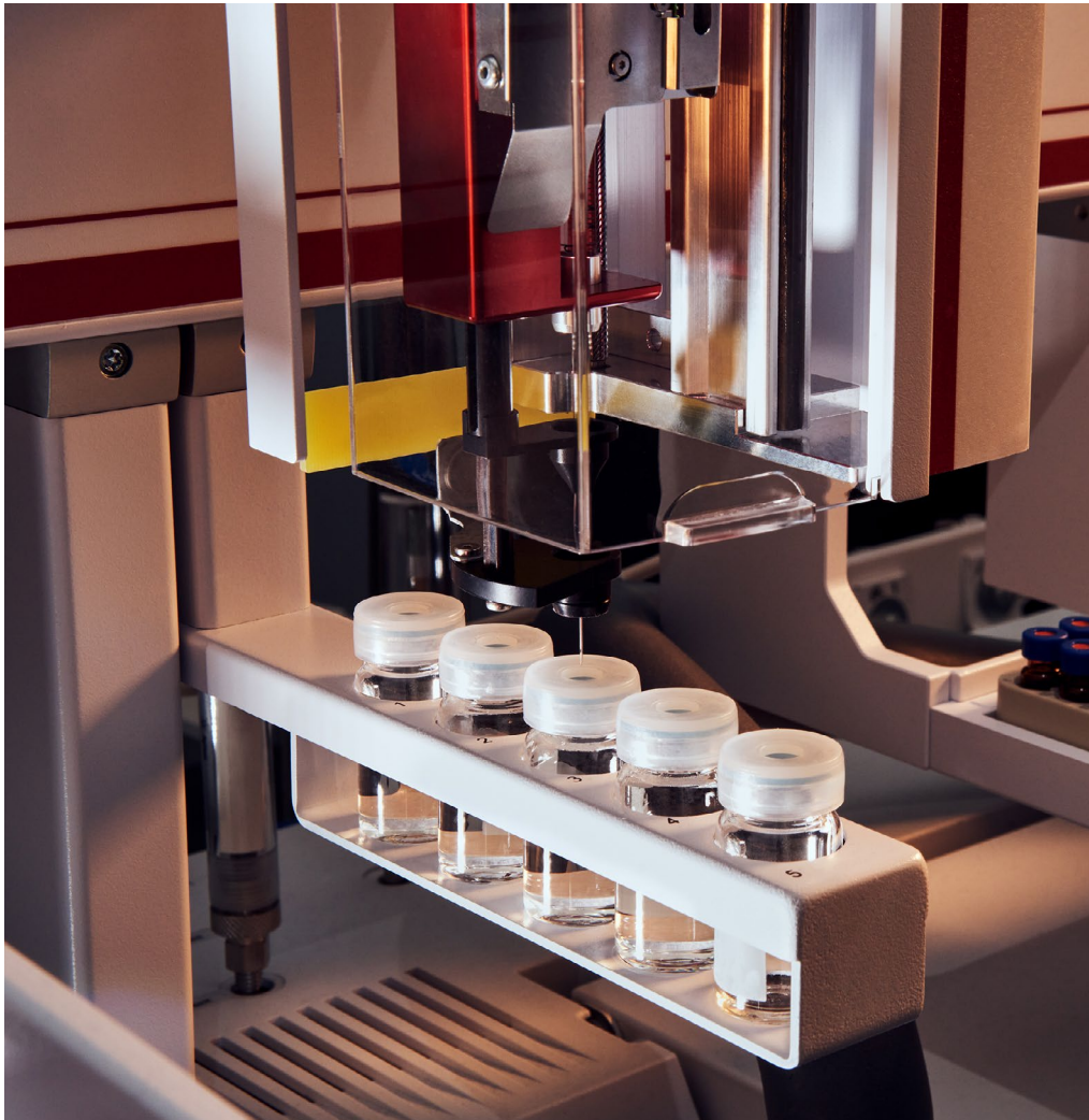
We evaluate materials for substances restricted in our Regulated Substances Specification — including VOCs — using equipment like this gas chromatography/mass spectrometry (GC/MS) system.
