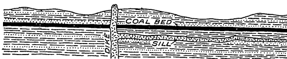
FIGURE 15.—Dike cutting coal bed and sill intruded in a position to affect the quality of the coal.
