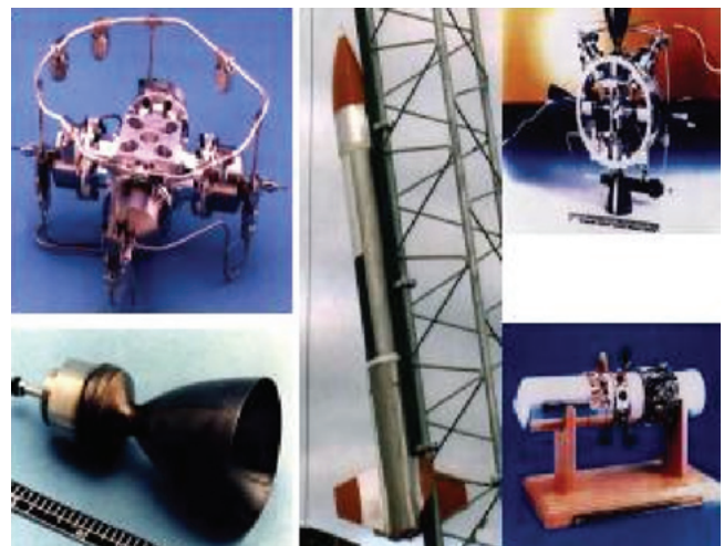
Astrid Flight Experiment Wet Mass: 209.4g Dry Mass: 8250g Prop. Mass: 12690g \Delta V > 2\text{km/s} Thrust > 450 N
