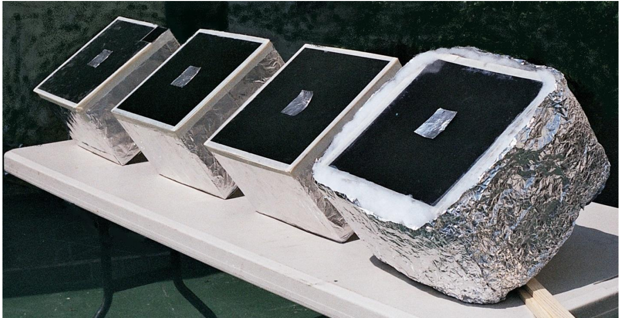
Picture 06: Verification of Robert Wood's Experiment - 1st Phase. Boxes aligned to the incoming solar irradiance. Notice the hole on the sheet of acrylic of the first box and the coating of white glass wool in the proximal box.
