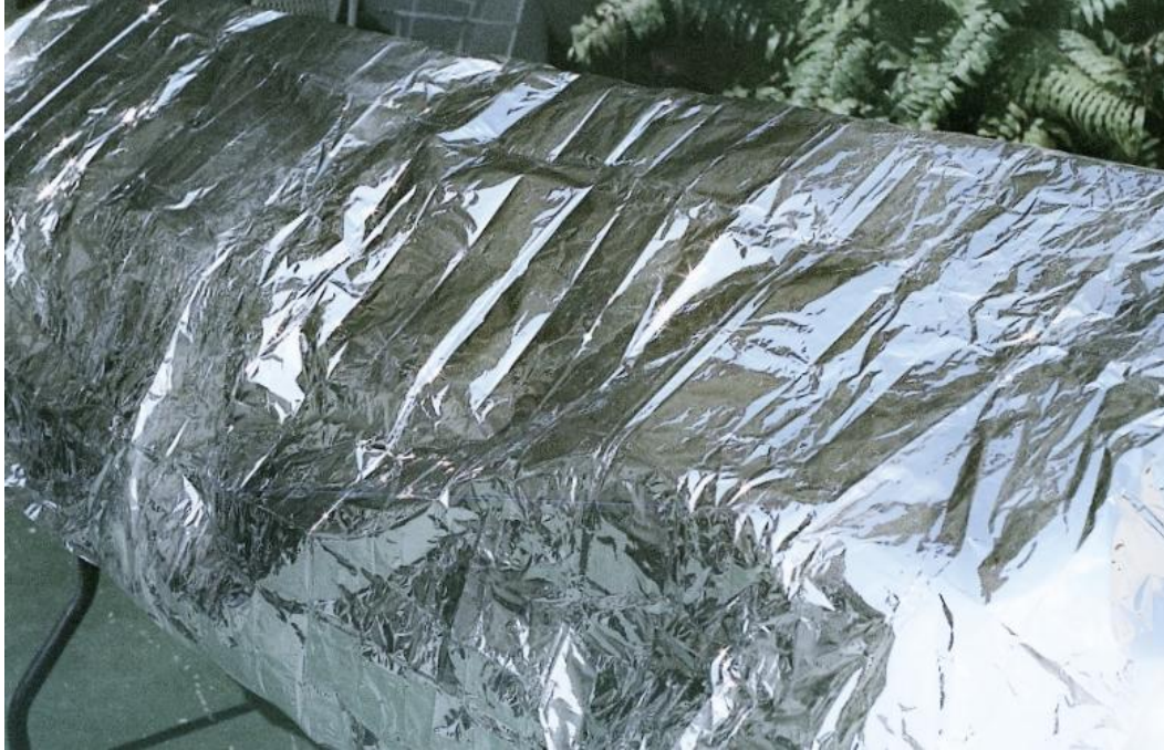
Figure 07: Verification of Robert Wood's Experiment - 1st Phase. Photograph of boxes protected by aluminum sheeting prior to testing
