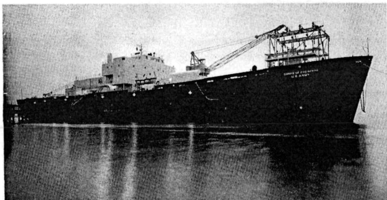
Figure 12 The Sturgis (MH-1A), a floating nuclear power plant, achieved criticality on January 25, 1967. In the diagram the power lines run off the bow into the region needing power. The center photograph shows the Sturgis moored at Fort Belvoir, Virginia. On the right one of the 32 fuel elements that compose the core of the Sturgis is lowered into place during fueling operations.
