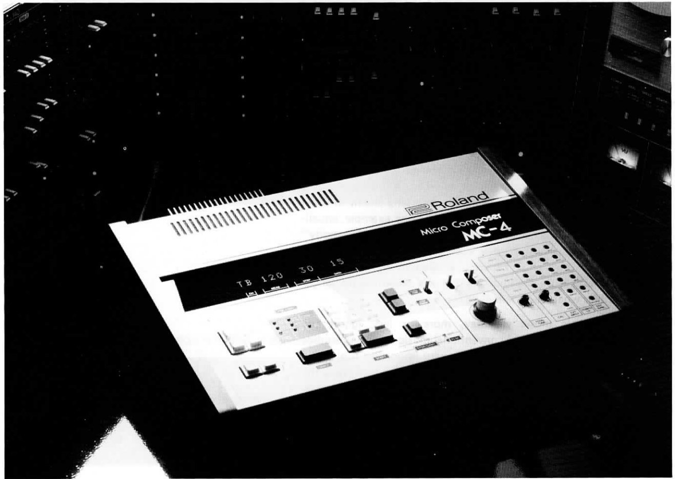
Fig. 3-32 Roland MC-4 MicroComposer (Computer Controller)
