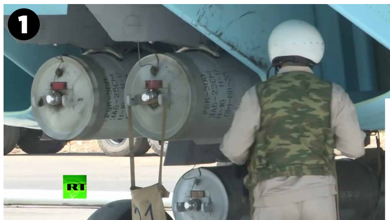
Image from RT video identifying cluster munition and incendiary cluster munition mounted on Russian attack aircraft (Source—RT/YouTube)
