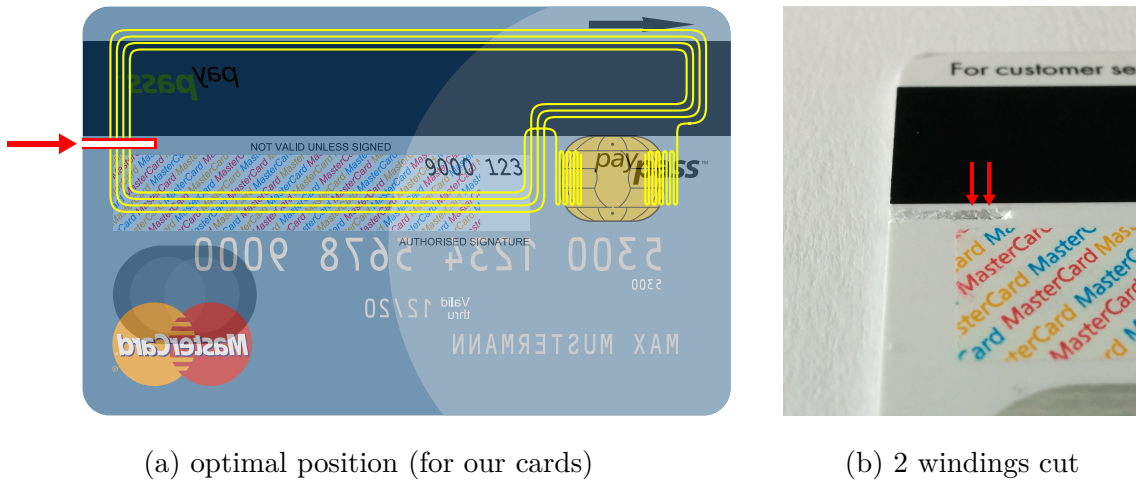
Figure 14: Optimal position to cut the antenna loops
