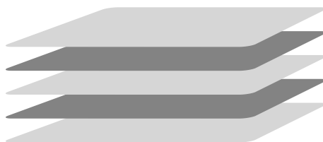
Figure 1: Stacked layers of a plastic card
