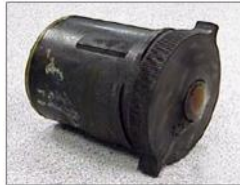
BATTERY COOLANT UNIT (BCU)
