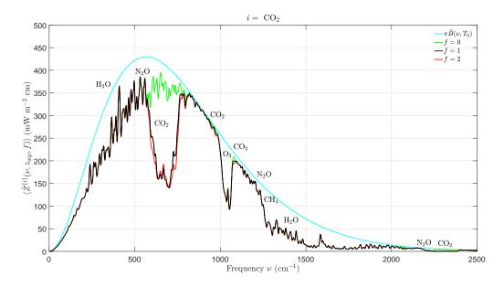
Figure 5: The spectral forcing at current levels of carbon dioxide,  $CO_2$ , (the black curve with f = 1), or if concentrations of carbon dioxide are doubled (the red curve with f = 2), or if all carbon dioxide is removed (the green curve with f = 0). See the caption of Fig. 4.
