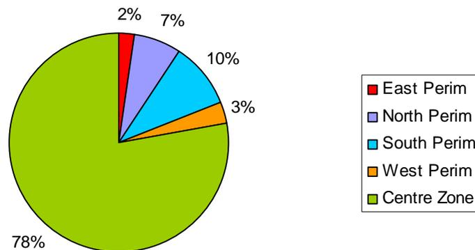
Figure 10. Zone cooling percentage breakdown
