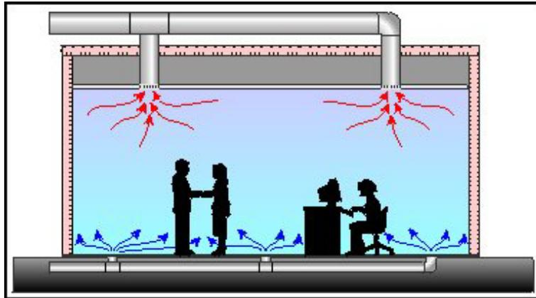
Figure 16. Displacement ventilation effects
