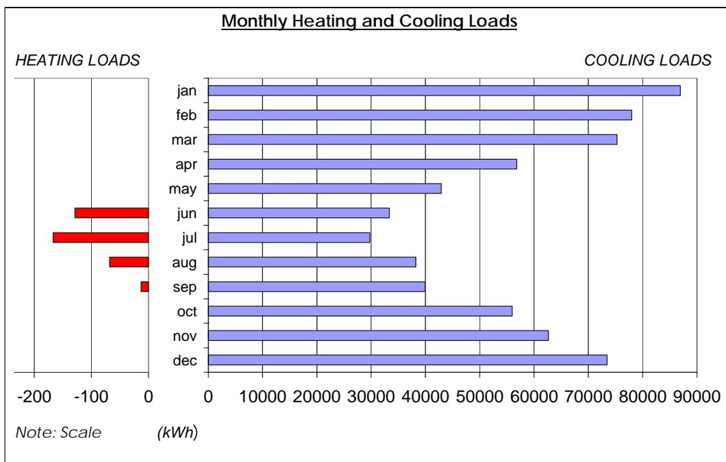
Figure 8. Monthly breakdown of heating and cooling requirements of total building
