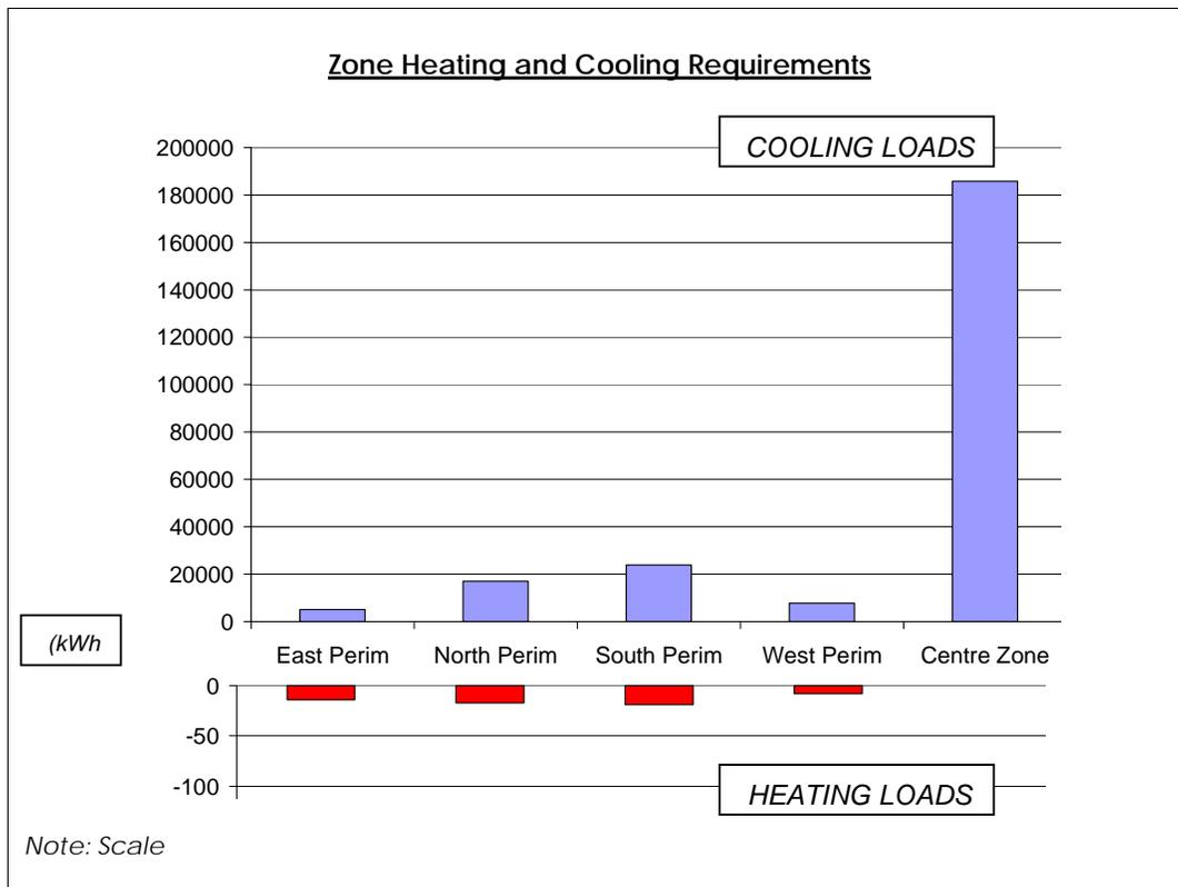
Figure 9. Zone breakdown of heating and cooling requirements
