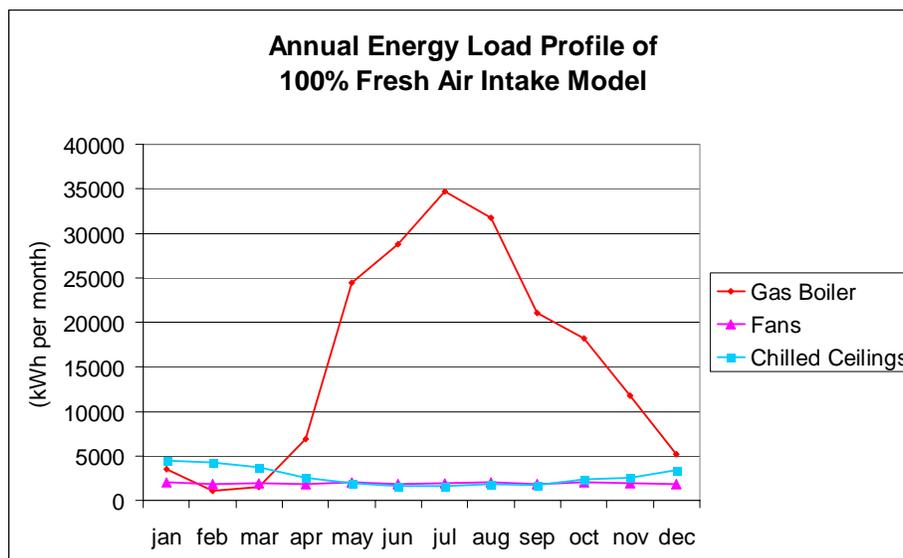
Figure 22. Estimated annual energy load profile for 100% fresh air model
