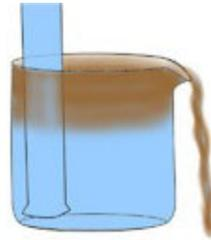
Figure 3. Displacement ventilation air layering effect
