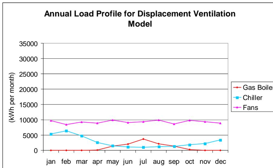
Figure 17. Estimated annual energy load profile for the displacement ventilation model
