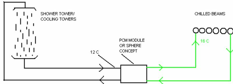
Figure 24. Basic Phase Change Material (PCM) schematic
