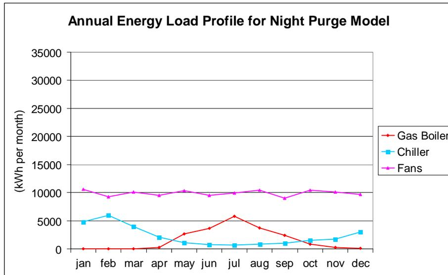
Figure 14. Estimated annual energy load profile for the night purge model
