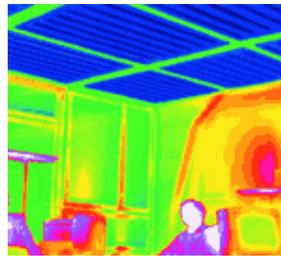
Figure 4. Chilled ceilings radiant cooling effects
