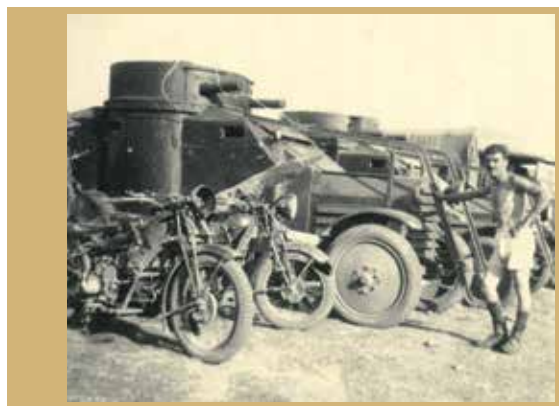
The Autobinda in service during World War I. This is the later version on the Tronchi chassis, identifiable by the single gun turret and exposed front wheels.
