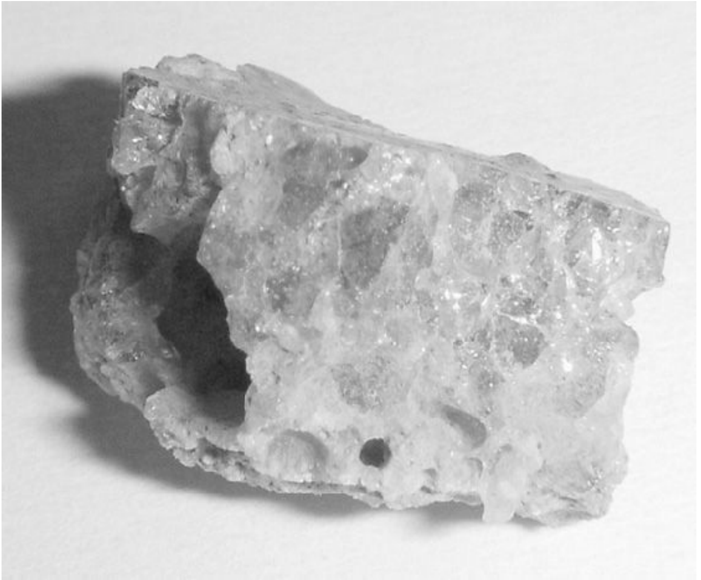
FIGURE 4. Trinitite, an entirely new mineral formed by the explosion of the Gadget, the first nuclear device. Photograph by Shaddack.
