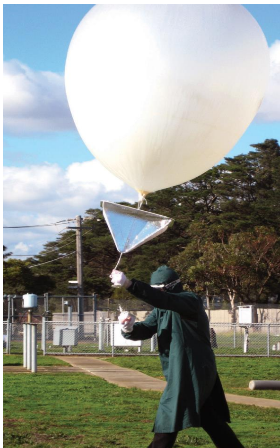
Photo 1 – Weather balloon and attachments, released by weather observer Photo credit: Bureau of Meteorology, 2009
