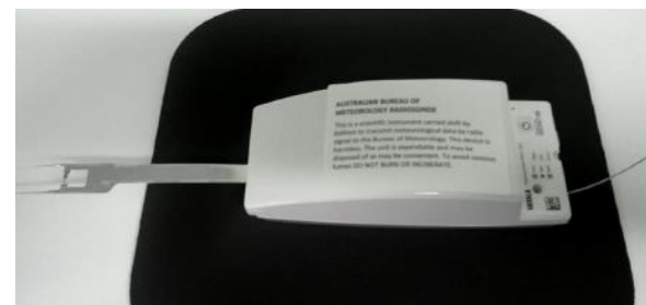
Photo 2 – Radiosonde, with Bureau label including how to dispose of radiosonde.
