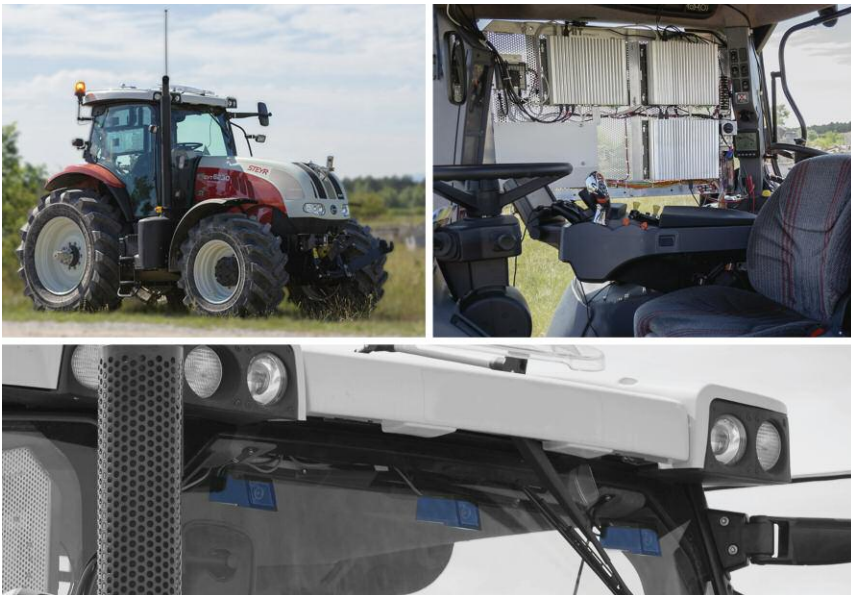
Figure 1: Top left: research platform Steyr 6230 CVT, Top right: additional computers running dedicated software (3x Intel i7 Ivy Bridge), Bottom: windshield mounted AIT stereo camera system (light blue).
