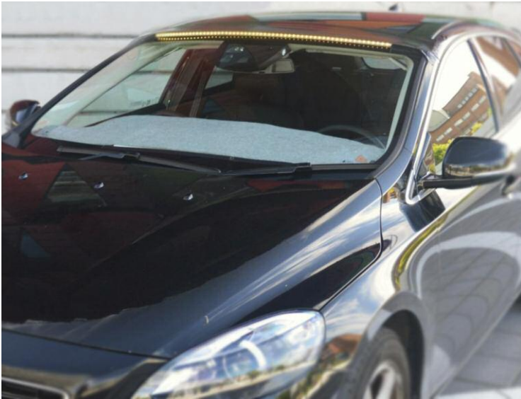
Figure 1: The AVIP concept. The changing LED light communicates the intention of an autonomous vehicle.
