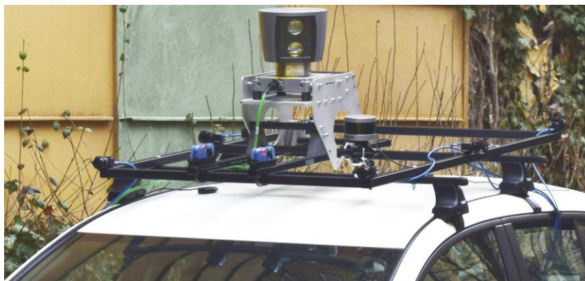
Figure 1: A host of image and range sensors are mounted onto the electric test car.
