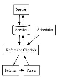
Figure 5: Overview of the architecture for the next-generation CollecTor.
