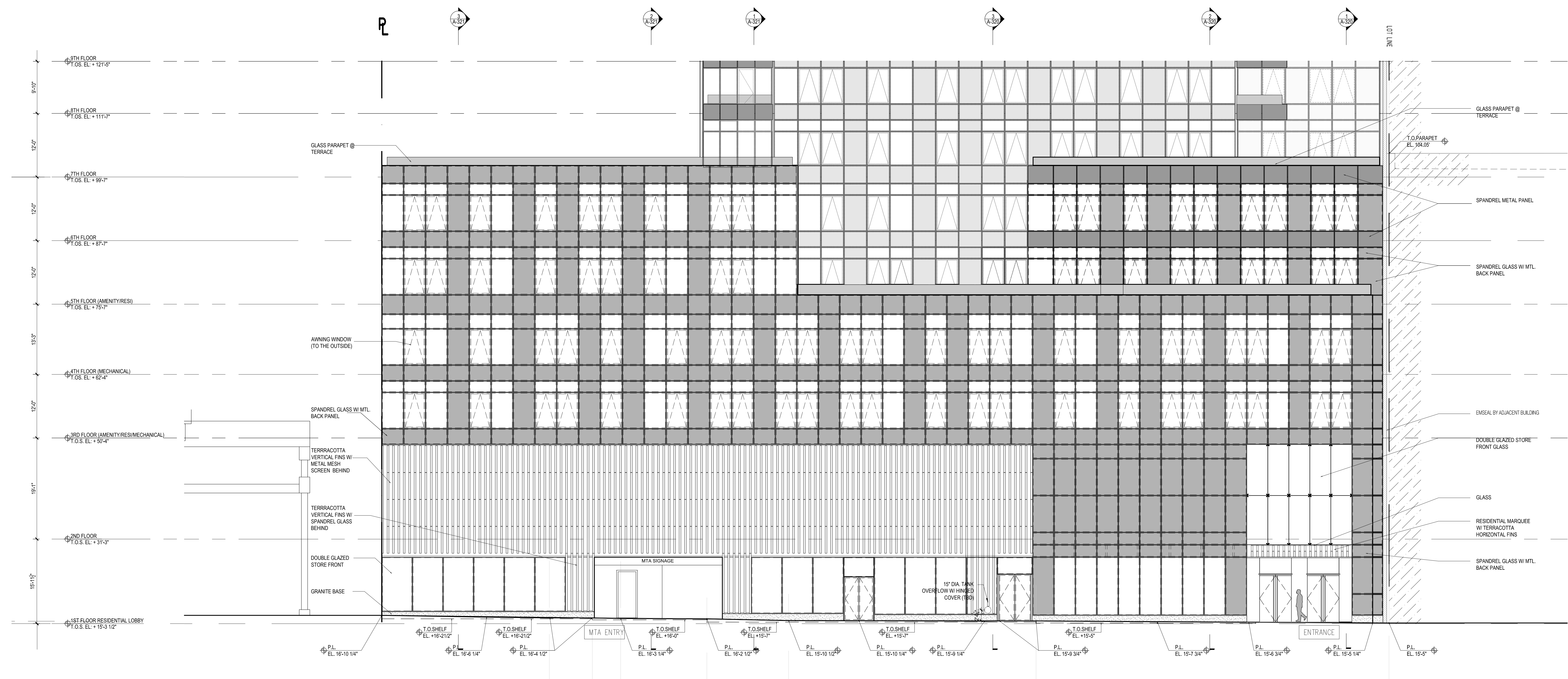
1 SOUTH BASE ELEVATION Scale: 1/8" = 1'-0"
