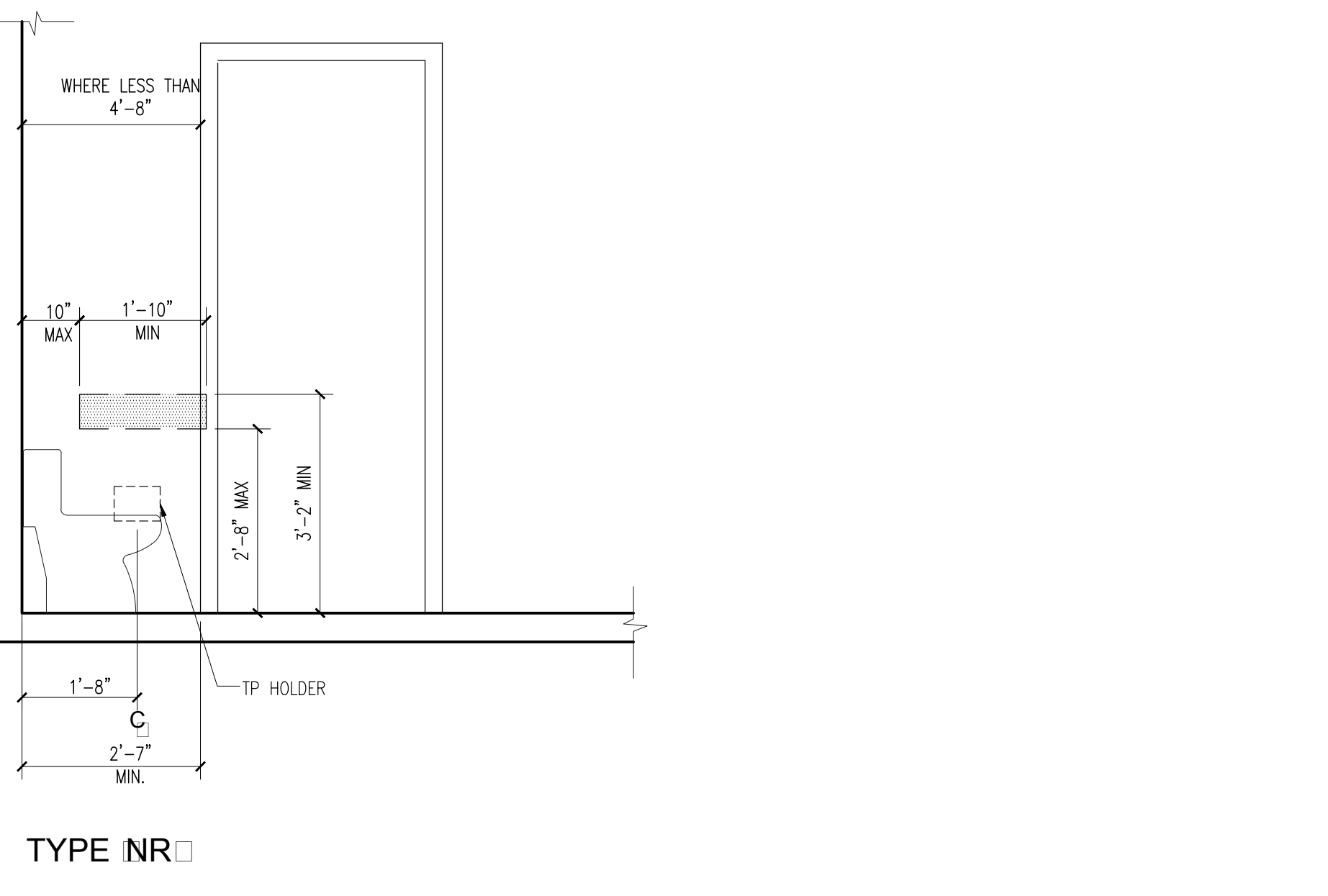
TYPE NR 6 Reinforced Areas & Requirements @ WC Scale: 1/2"=1'
