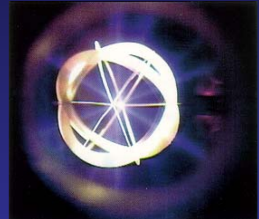
IEC-PSI at 5 \times 10^6 n/s (D-D)
