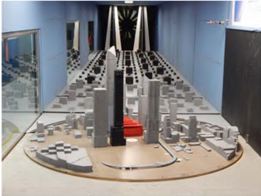
Figure 2.1b – Wind tunnel proximity models for test configuration C2
