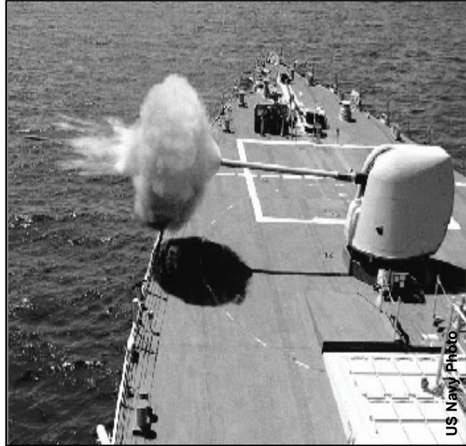
Figure D-2. USN MK45 lightweight gun system
