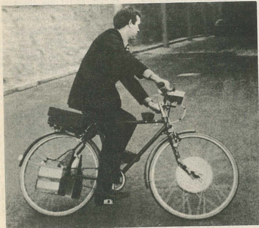
Front-drive electric bicycle has synchronous motor and gearbox integrated in front hub. Top speed is 18 mph in prototype form; range is up to 40 miles
