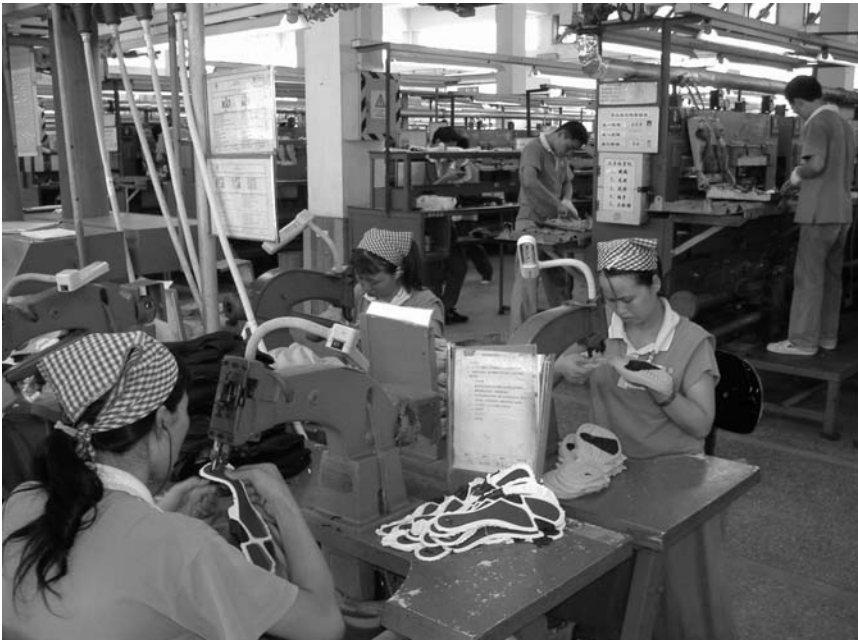
Figure 6—Workers in the Hot Press Department, where operators of “skiving” machines (foreground) trimming rubber soles are immediately adjacent to hot presses generating noise exposures above 90 decibels and temperatures above 35 degrees Centigrade.
