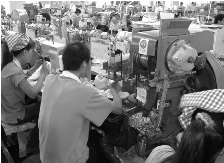
Figure 3—Lean production cell where a punch-press operator installing metal eyelets wears hearing protection for noise levels in the 87–89-decibel range, but the immediately adjacent sewing machine operators are unprotected against these noise exposures.
