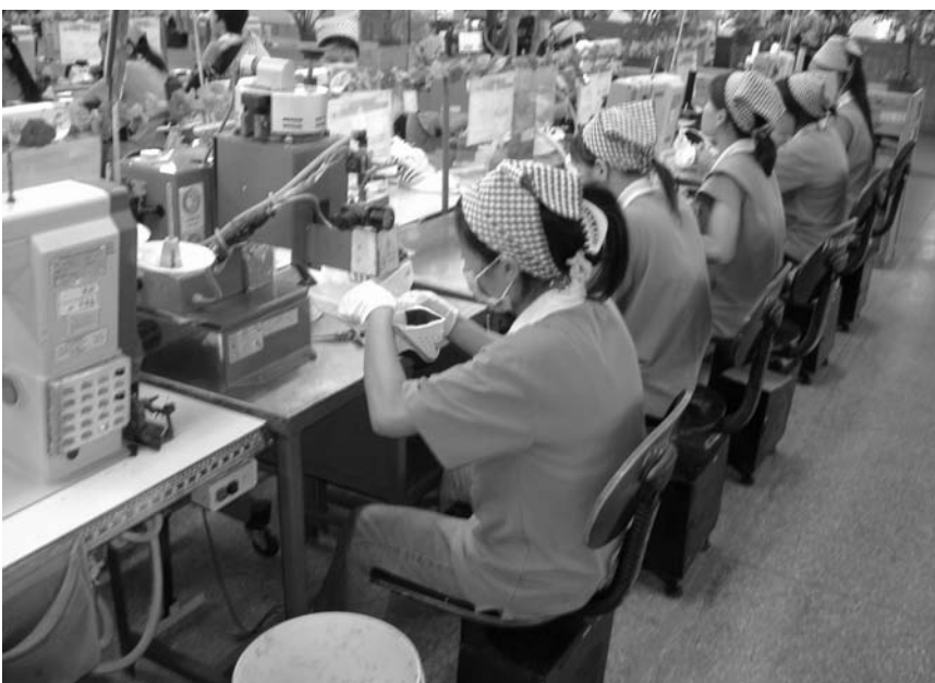
Figure 4—Lean production cell where a worker applying heated spray adhesive is wearing a cloth “respirator” (which offers no real protection) while immediately adjacent workers assembling parts and operating sewing machines are exposed to airborne contaminants without any ventilation or protective equipment.
