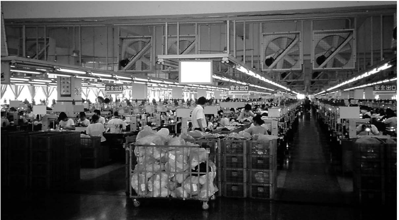
Figure 1—Traditional assembly production in 2000 at a sports shoe factory in Dongguan City where 2,000 women sit behind sewing machines in the fifth-floor Stitching Department assembling components of the upper shoe. The sewed parts are warehoused until they are assembled in the fourth-floor Stockfit and Assembly departments, then sent on to the third-floor inspection and packaging departments. All photo credits: Garrett Brown.
