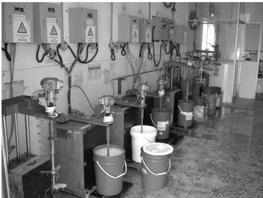
Figure 7—Chemical mixing department of the factory's chemical warehouse, where adhesives and solvents are mixed in open processes without any controls. In May 2006 technicians from the Chinese Center for Disease Control conducted direct-reading instrument screening of the area and found concentrations of n-hexane to be 4.5 times the Chinese eight-hour time-weighted average exposure limit (446 parts per million vs. the 100 ppm limit).
