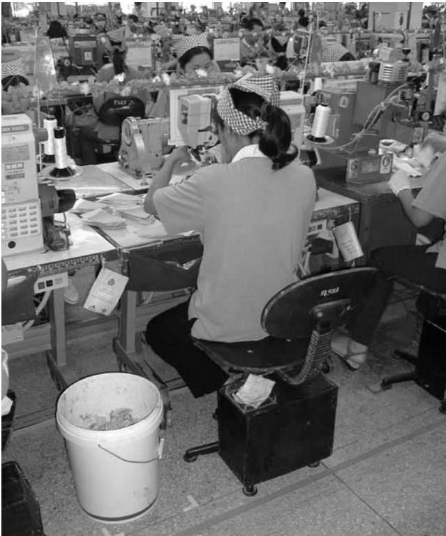
Figure 8—Non-adjustable stools used throughout the 13,000-worker factory, which provide no support or protection against ergonomic hazards.
