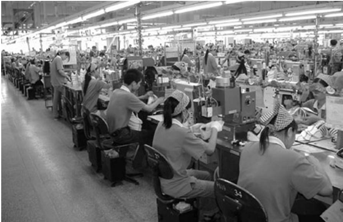
Figure 2—Lean production cell in the studied factory in 2006 where workers sitting next to one another sew components, spray adhesive onto parts, install eyelets, and assemble and inspect the final product. The close proximity of these different operations means workers are simultaneously exposed to chemical and noise hazards.
