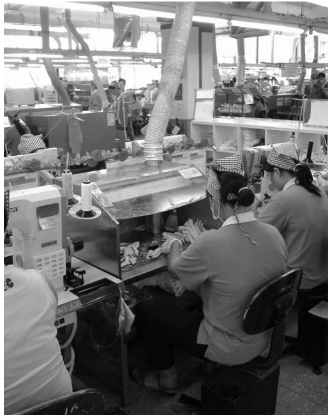
Figure 5—Lean production cell where a local exhaust ventilation (LEV) system has been installed to control airborne solvent and adhesive vapors. Such systems must be carefully designed, maintained, and periodically tested to ensure that air flow rates actually capture vapors and remove them from workers' breathing zones. The worker here is also wearing a cloth "respirator," possibly indicating she is still exposed to discernable levels of airborne contaminants.
