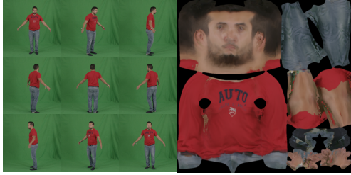
Figure 4. We back-project the image color from several frames to all visible vertices to generate a full texture map.
