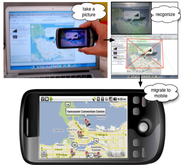
Figure 1. A user takes a picture of the screen of her computer and then sees the application with the current state on her phone. Our system recognizes the application that the user is looking through the camera, automatically migrates it onto the mobile phone, and recovers its state.
