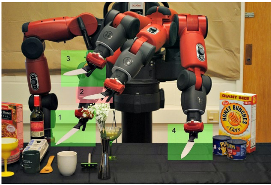
Fig. 1: Zero-G feedback: Learning trajectory preferences from suboptimal zero-G feedback. (Left) Robot plans a bad trajectory (waypoints 1-2-4) with knife close to flower. As feedback, user corrects waypoint 2 and moves it to waypoint 3. (Right) User providing zero-G feedback on waypoint 2.
