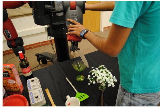
Fig. 1: Zero-G feedback: Learning trajectory preferences from suboptimal zero-G feedback. (Left) Robot plans a bad trajectory (waypoints 1-2-4) with knife close to flower. As feedback, user corrects waypoint 2 and moves it to waypoint 3. (Right) User providing zero-G feedback on waypoint 2.
