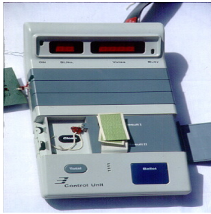
Closing the inner door with thread ECIL Machine
