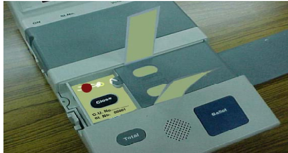
Sealing the inner door with Special Tag ECIL Machine
