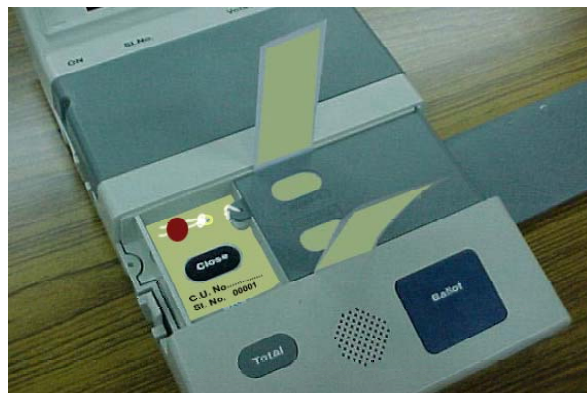
Sealing the inner door with Special Tag BEL Machine
