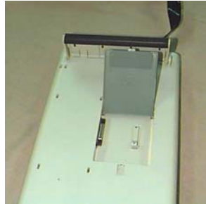
Socket for linking one Ballot Unit with the other Ballot Unit at the Back of Ballot Unit
