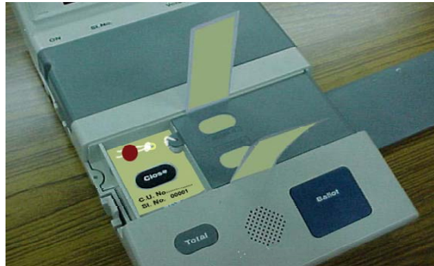
BEL Machine Sealing the inner door with Special Tag ECIL Machine
