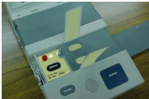
Sealing the inner door with Special Tag
