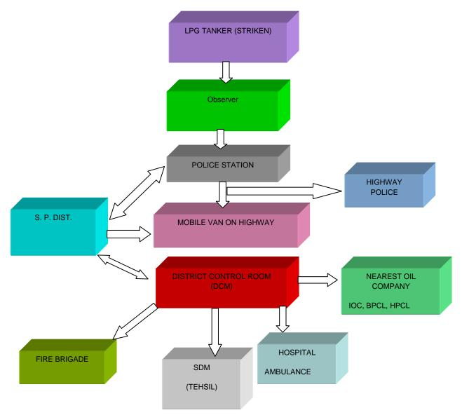
Below is the Flow chart in case of LPG Leakage
