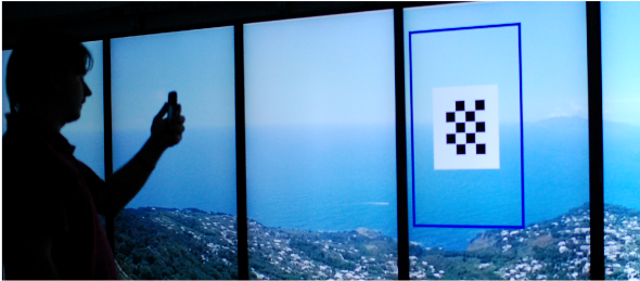
b) The barcode, once identified, changes to a checkerboard marker that continuously shifts as the user orients the phone toward a target position, as if it were projected from the phone.
